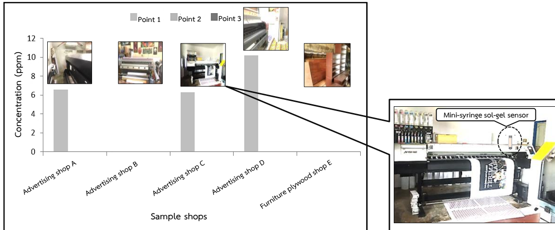
Figure 8 The relationship between formaldehyde concentration and sample shops. (Inset: The installing point of the mini-syringe formaldehyde sol-gel sensor inside the shop)
