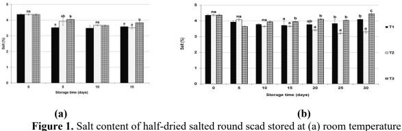
**`igure 1.** Salt content of half-dried salted round scad stored at (a) room temperatur and (b) chilling condition under air (T1), vacuum (T2) and air with oxygen absorber (T3) packaging
