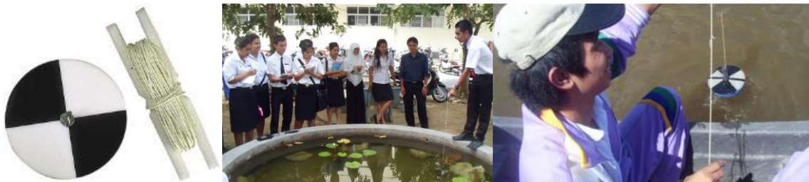
Fig. 4 Secchi disk and using practice by student
