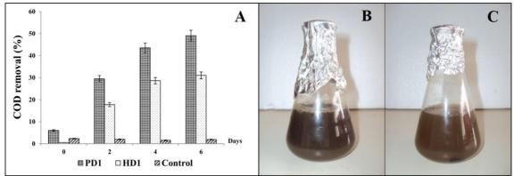
Figure 4Comparison of (A) COD removal from *Aspergillus* sp. PD1 and *Aspergillus* sp. HD1and comparison of (B) before treatment and (C) after treatment from enzymeproducing fungi *Aspergillus* sp. PD1 cultivation in palm oil mill effluent on a shaker (200 rpm) at 45°C for 6 days.
