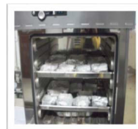
Figure 7: Determination of percentage of dried latex according to the standard method.
