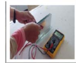
Figure 5: Then measure the capacitance with a multimeter and an LRC
