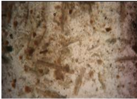
Figure.2 Characteristics of bagasse that was treated using a was selected and add 2.5 Unit cellulase enzyme for 60 minutes.
