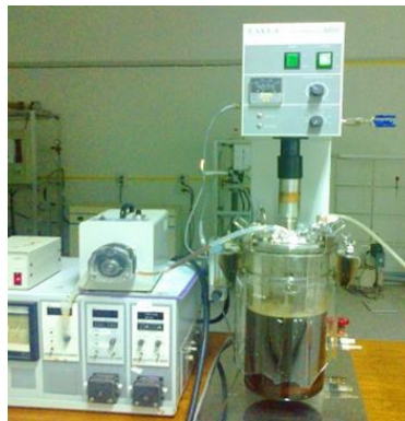
Figure 1. The Ethanol fermentation with Saccharomyces sp.TISTR 5091 from bagasse that has been treated
