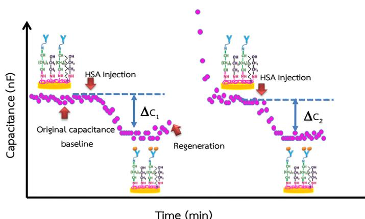
**Figure 2** Flow injection capacitive immunosensor system using PpPD modified electrode for the detection of HSA.
